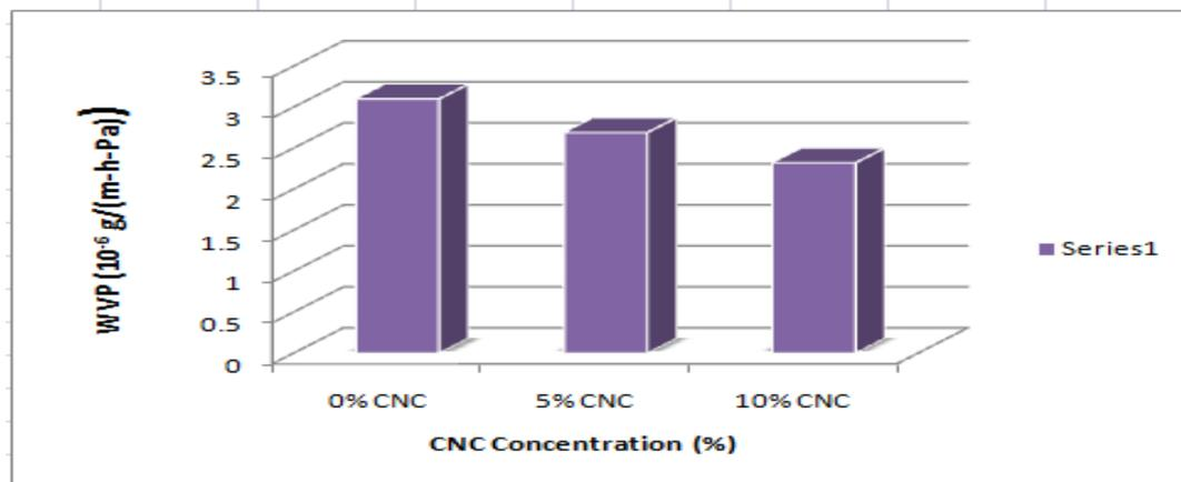
Fig. 3.4: Water vapour permeability of nanocomposite films
