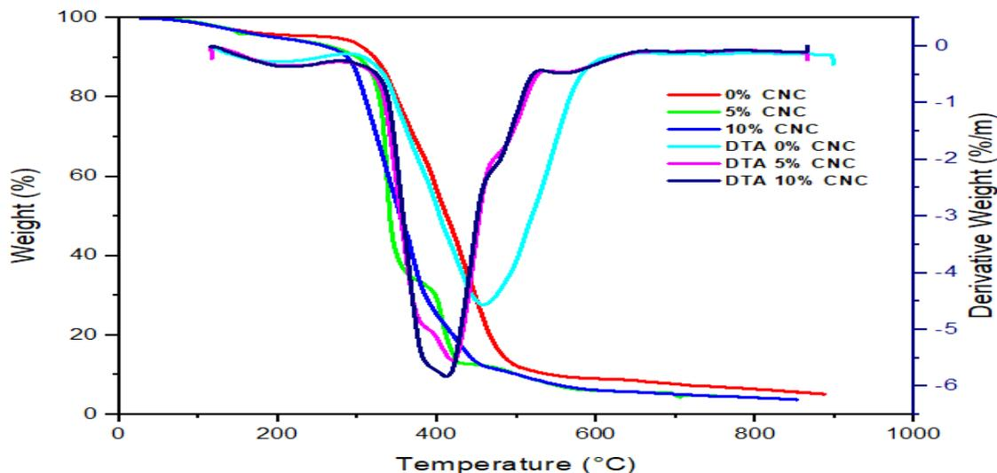
Fig. 3.6: Thermal decomposition of 0wt%, 5 wt% and 10 wt% CNC
