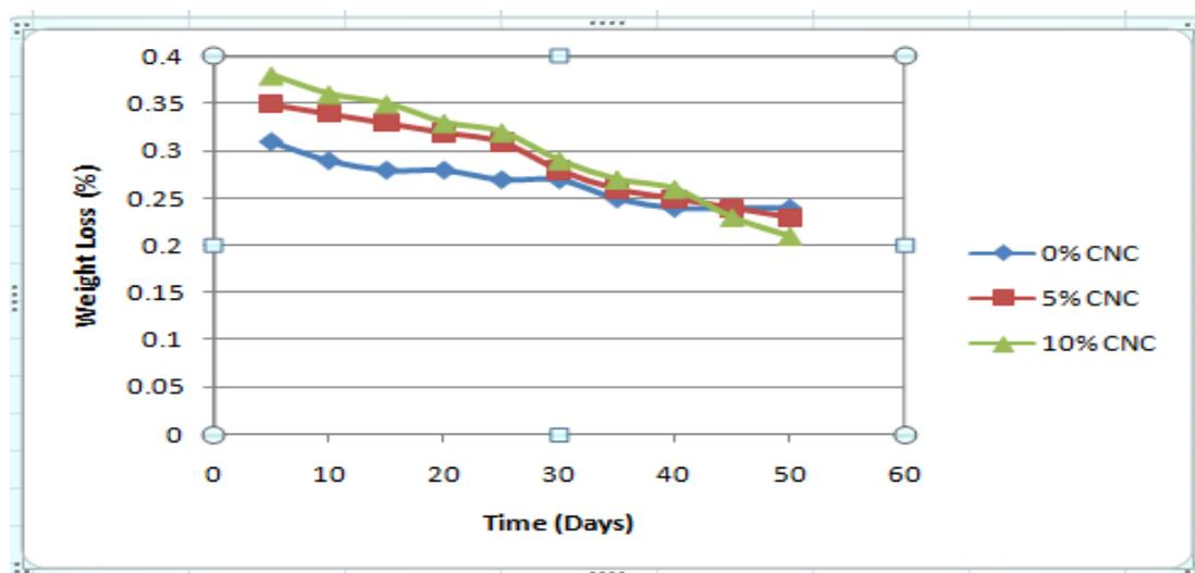
Fig. 3.5: Soil degradation of the nanocomposite films
