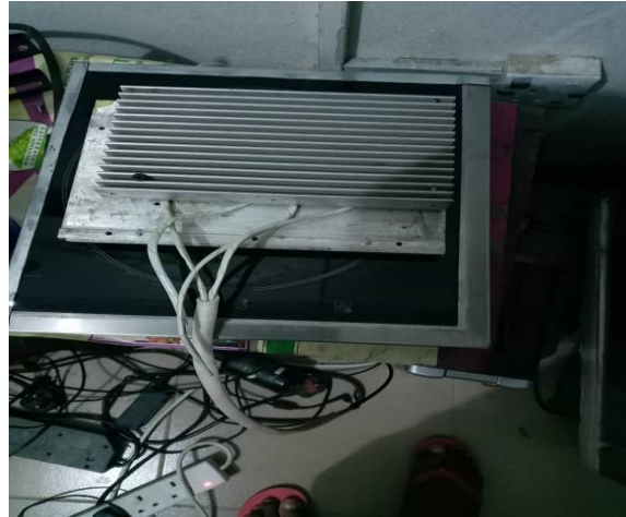
Fig 2.1:2 Series TEG connection with out plate experiment set up (Field of authors)
