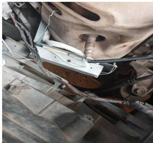
Fig 2.2 TEG series connection and Manifold Experiment setup (Field of Authors)
