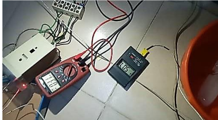
Figure 3: Picture of experimental setup of the Design, characterization, coupling and calibration of a type-k thermocouple (Source: Field of authors)
