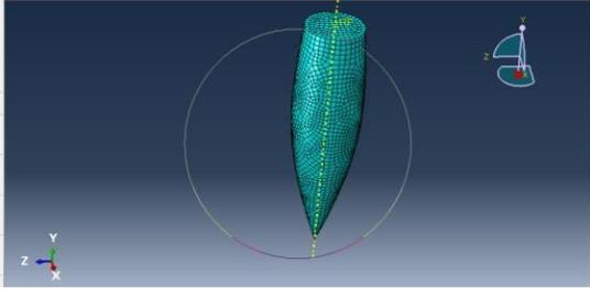
**Figure 3:** Meshed Conical Projectile
