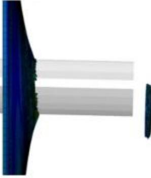
**Figure 6:** Circular Plug Ejection of Blunt Projectile
