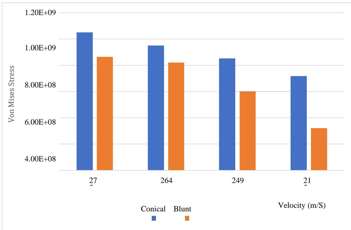
**Figure 5:** Chart of Von Mises Stress Comparison between Conical and Blunt Projectile
