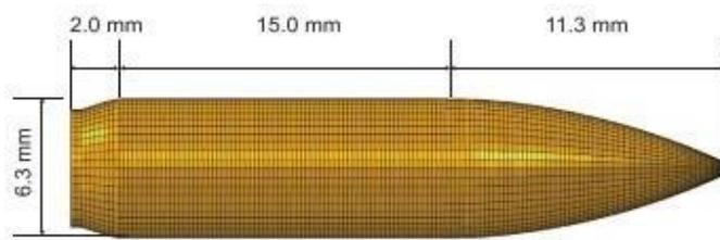
**Figure 2:** Model of the Conical Projectile and Dimensions
