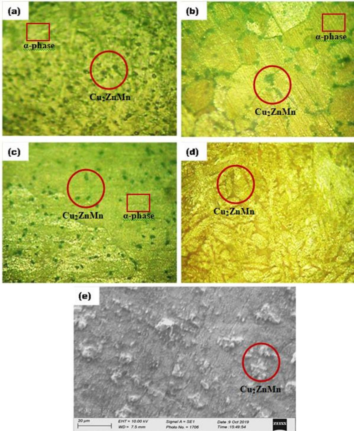
**Figure 3: Optical micrograph (a) Cu-20Zn (b) Cu-20Zn-0.1Mn (c) Cu-20Zn-0.3Mn (d) Cu-20Zn-0.5Mn (e) SEM of Cu-20Zn-0.5Mn.**
