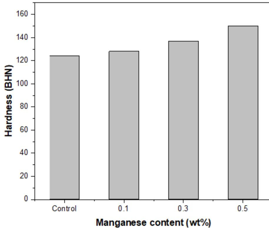
Figure 1: Effect of manganese content on the hardness of Cu-20wt%Zn alloy
