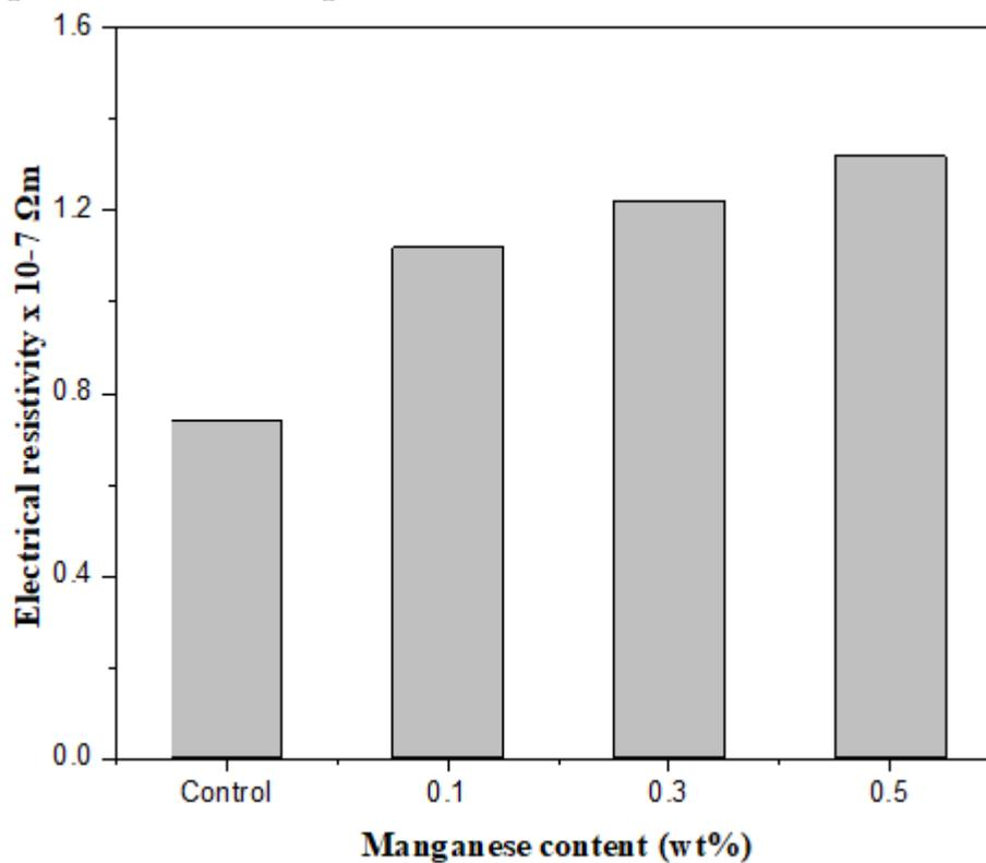
Figure 2: Effect of manganese content on the electrical resistivity of Cu-20wt%Zn alloy
