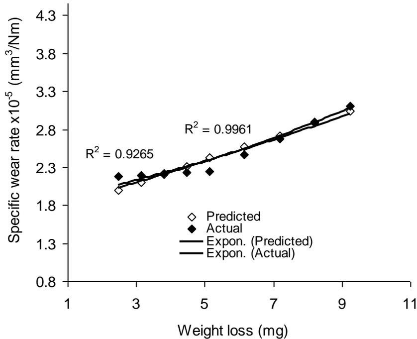
Figure 6: Coefficient of determination between specific wear rate and weight loss as evaluated from actual results and derived model
