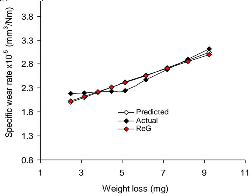
Figure 4: Comparison of specific wear rates of glass fibre-epoxy resin composite (relative to weight loss) from actual results, derived model and regression model.
