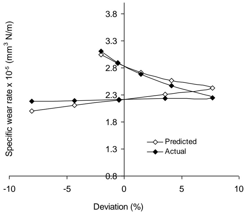
Figure 7: Variation of model-predicted specific wear rate of glass fibre-epoxy resin composite with its corresponding deviation from experimental results
