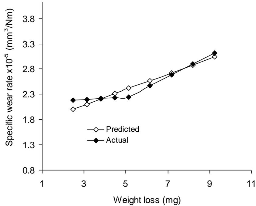
Figure 3: Comparison of specific wear rates of glass fibre-epoxy resin composite (relative to weight loss) from actual results and derived model.
