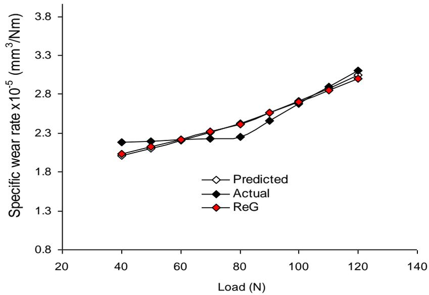
Figure 2: Comparison of specific wear rates of glass fibre-epoxy resin composite (relative to applied load) from actual results, derived model and regression model
