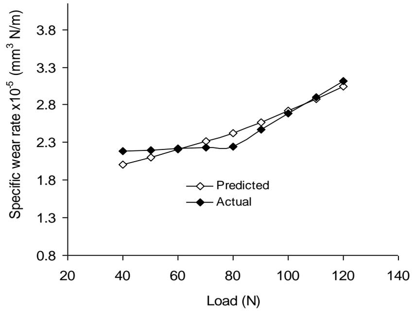
Figure 1: Comparison of specific wear rates of glass fibre-epoxy resin composite (relative to applied load) from actual results and derived model
