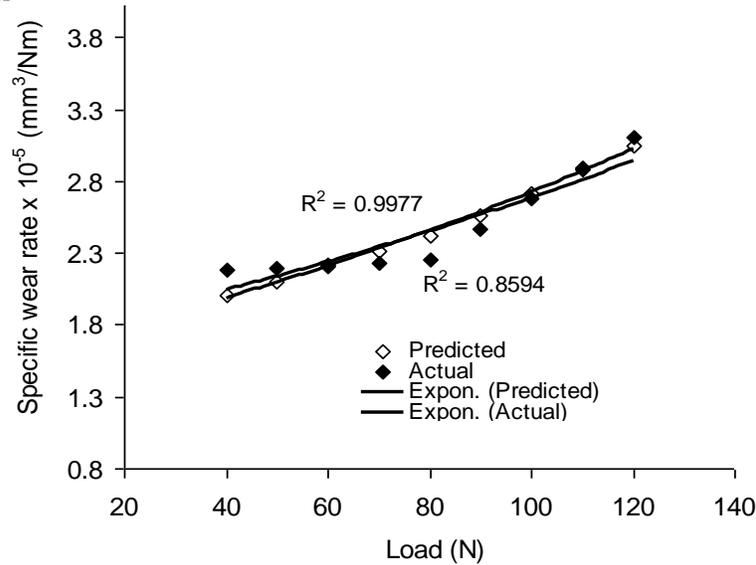
Figure 5: Coefficient of determination between specific wear rate and applied load as evaluated from actual results and derived model
