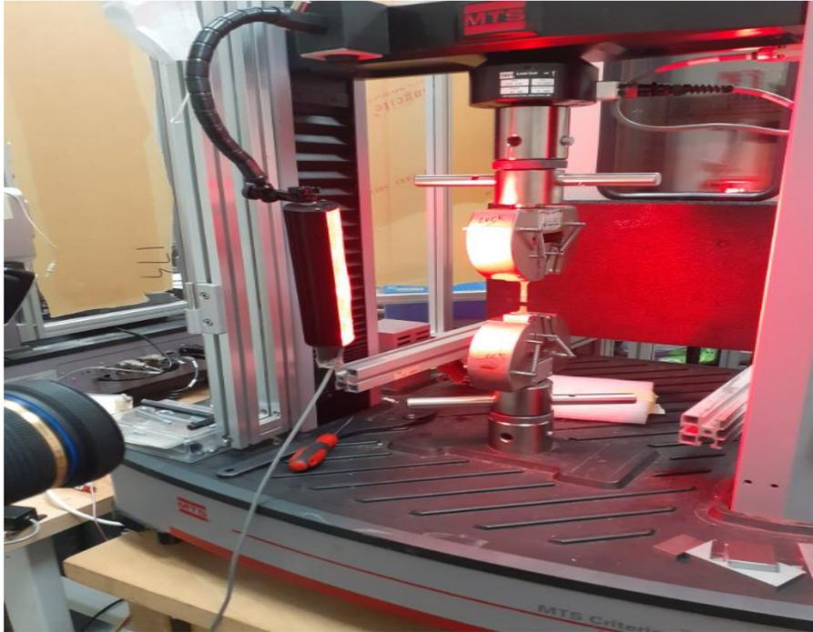
Figure 3. PA12 composite sample specimen between the lower base and upper fixture which had undergone uniaxial cyclic testing.
