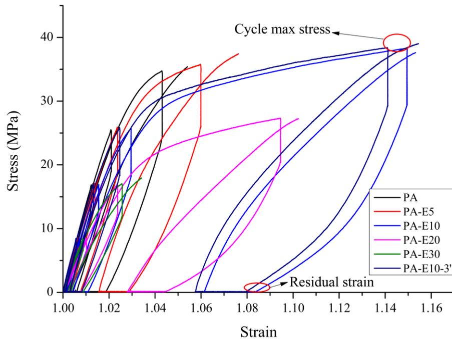
Figure 4. A schematic curve for the area of hysteresis loop, maximum stress, and residual strain for binary composites
