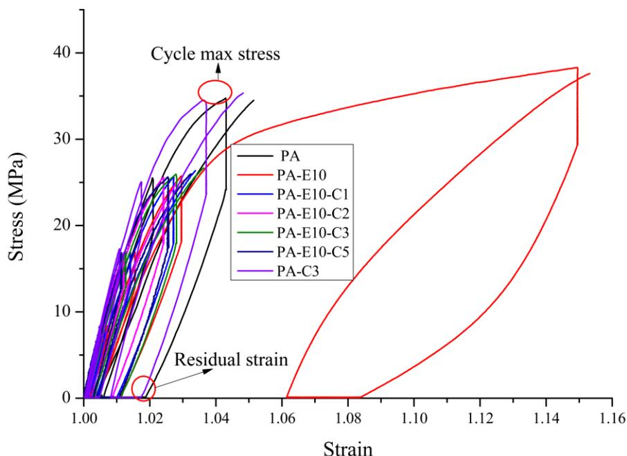
Figure 5. A schematic curve for the area of hysteresis loop, maximum stress and residual strain for binary/ternary nanocomposites
