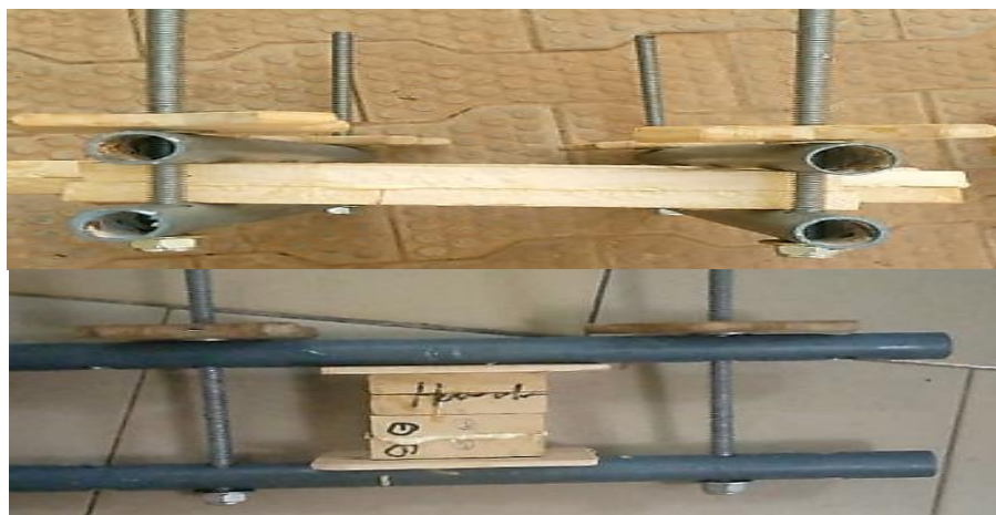
Figure 2: Improvised clamping device for pressure application
