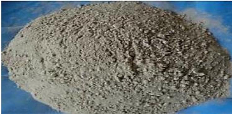
**Plate 1: Cement Kiln Dust**
