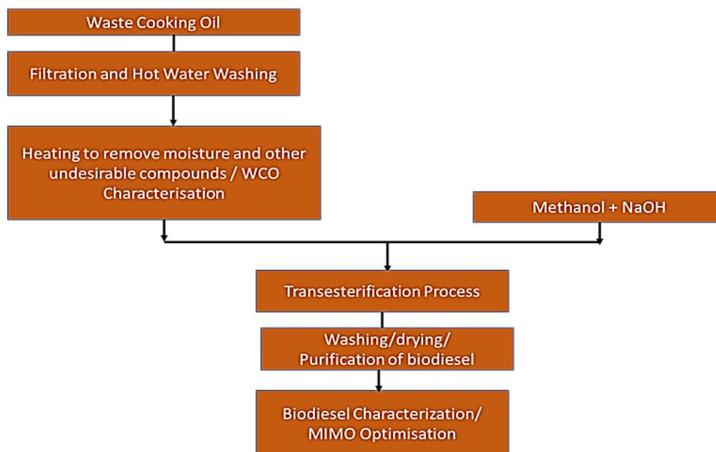
Figure 2: Biodiesel production and Optimization steps.
