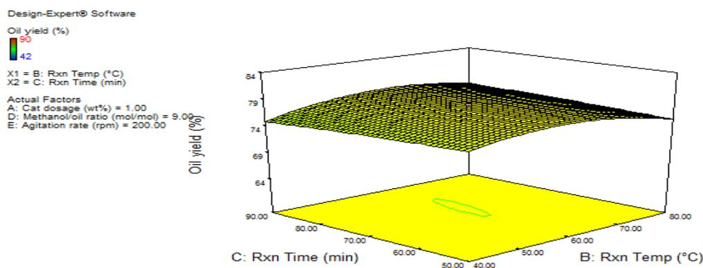
Figure 4a: 3D surface diagram of reaction time, reaction temperature and Biodiesel yields
