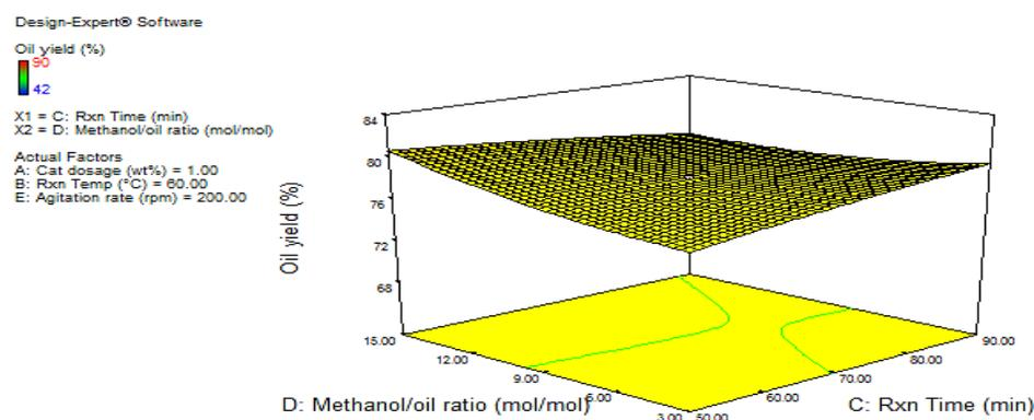
Figure 4c: 3D surface diagram of methanol: oil ratio, reaction time and Biodiesel yields
