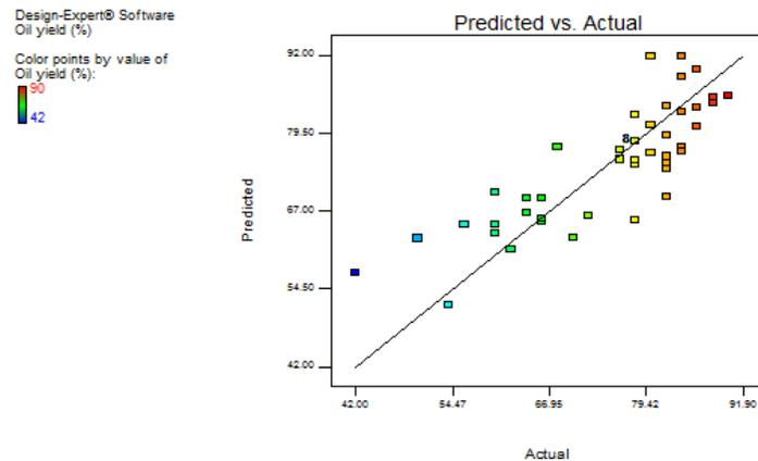
Figure 3: Plot of predicted values versus experimental values for the WCO biodiesel yield.
