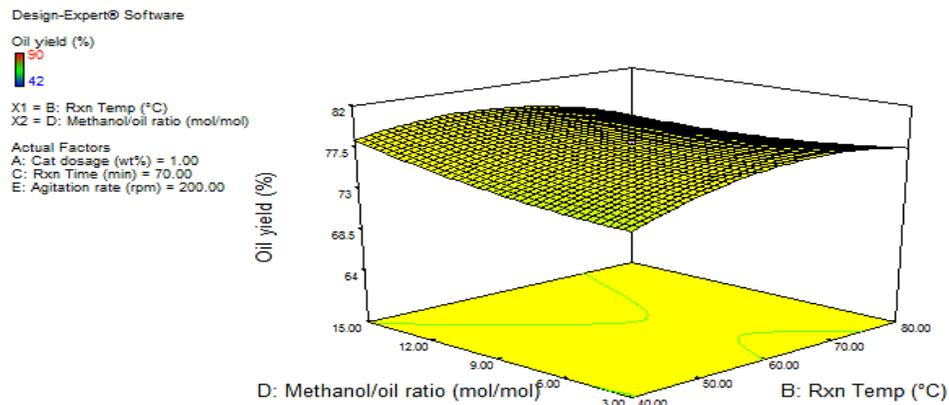
Figure 4b: 3D surface diagram of methanol: oil ratio, reaction temperature and Biodiesel yields
