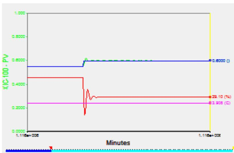
**Figure 13: Response of step change in methane fraction: Increase in methane fraction set point produce quick recovery by reducing the valve opening.**
