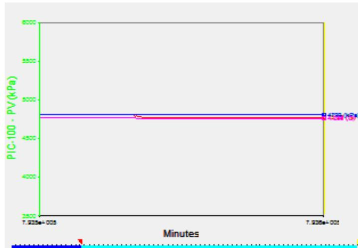
**Figure 8: Response of vessel pressure: The step change in molar flow shows no effect on Vessel pressure.**
