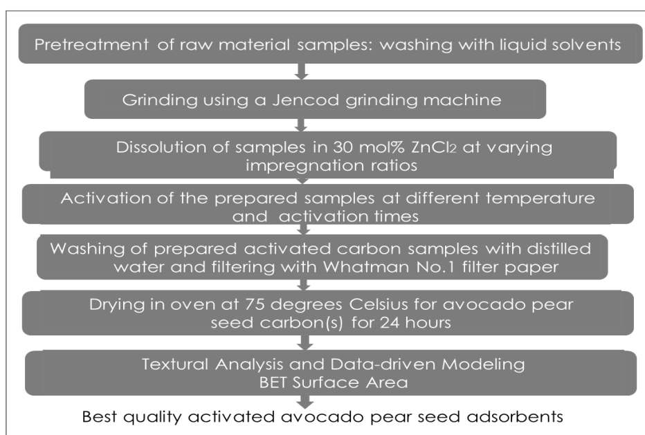
Figure 1: Diagrammatic illustration of the zinc chloride modified avocado pear seeds production process.
