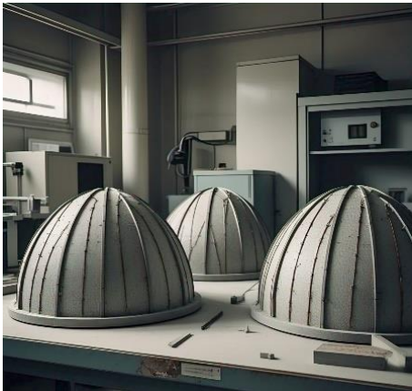
Plate 1: Three prototype shell structures fabricated using a combination of CFRP reinforcement and high-strength concrete.
