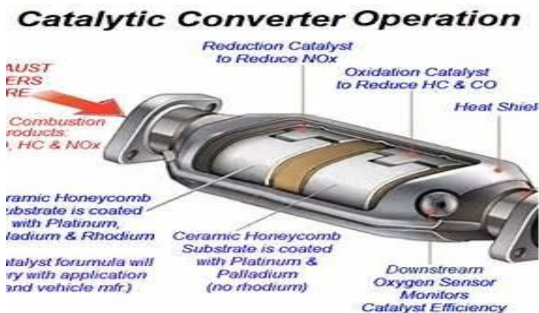
Figure 2: Catalytic converter operation
