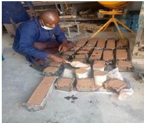
Plate 1. Preparation of geopolymer concrete samples
