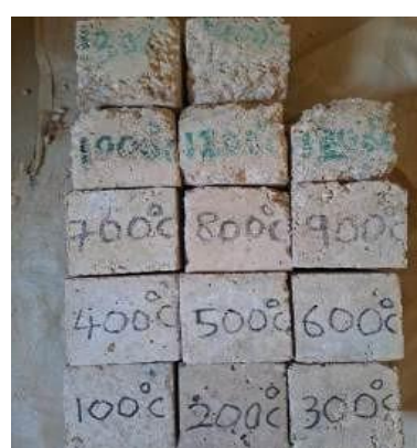
Plate 7. Samples after subjected to elevated temperature.
