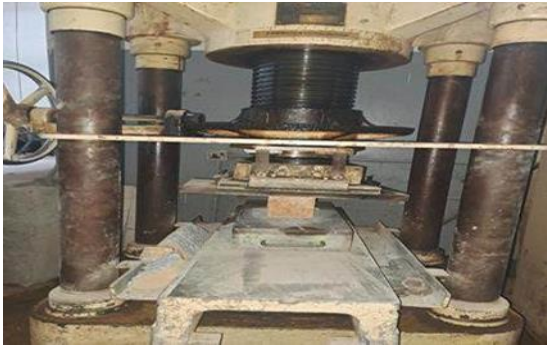
Plate 3. Compressive strength test in progress
