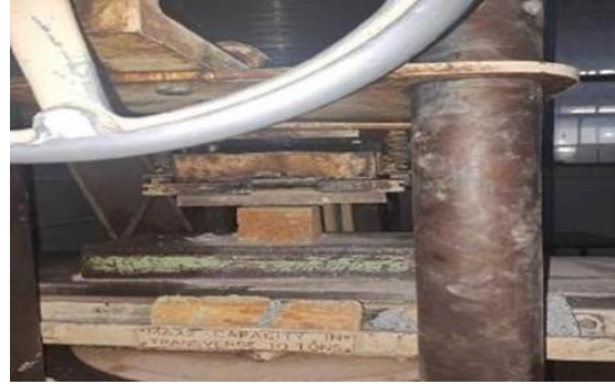
Plate 4. Crushed geopolymer concrete cube
