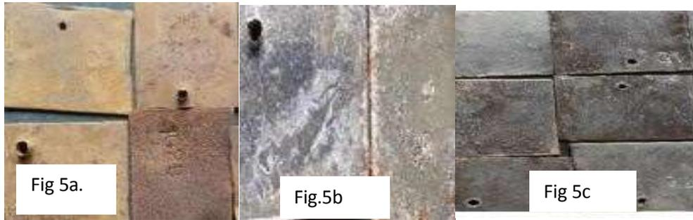
Figure 5a is uncoated sample subjected to corrosion, figure 5b is coated sample subjected to corrosion while figure 5c coated sample that was not subjected to corrosion.
