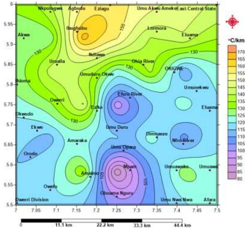
Figure 15: The geothermal gradient map over the area
