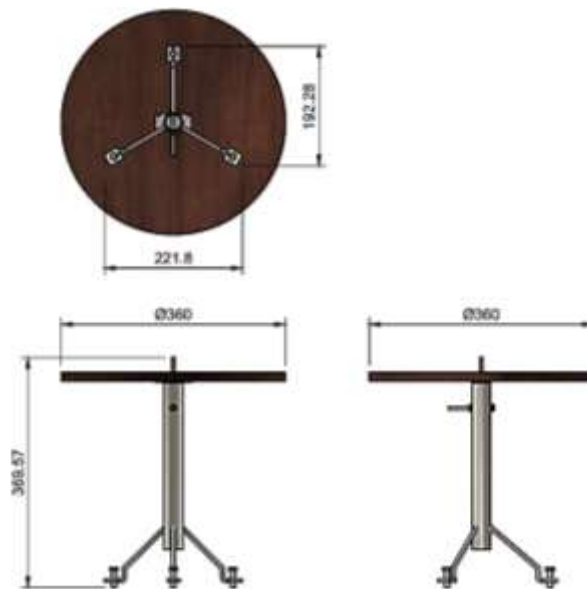
Figure 1: 2-D Representation of the Developed Force Table
