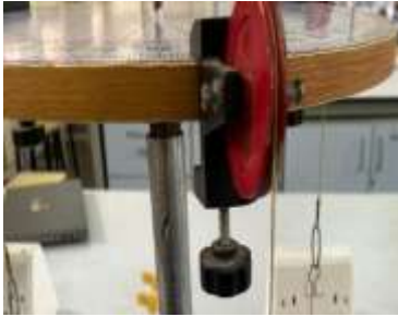
Figure 5: Pulley attached to Force Table
