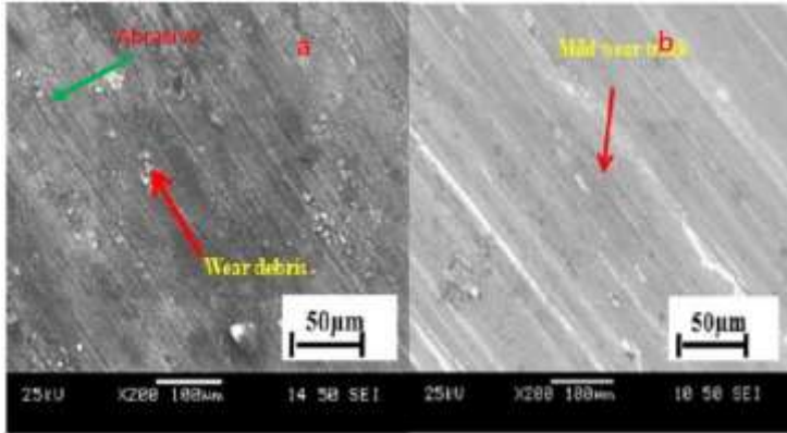
Figure 2: SEM Micrographs of the Worn Surfaces (a) Al 3 and (b) Al 7 Alloy b. Microstructure of the Aluminium Alloy
