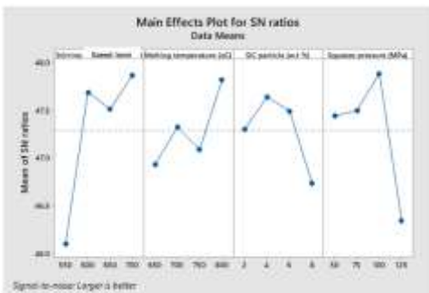
Figure 4: Main Effect Plot for Tensile Strength Test Figure 5: Main Effect Plot for Hardness Test
