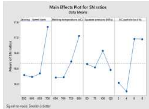
Figure 7: Main Effects Plots for S/N Ratio of Wear Rate
