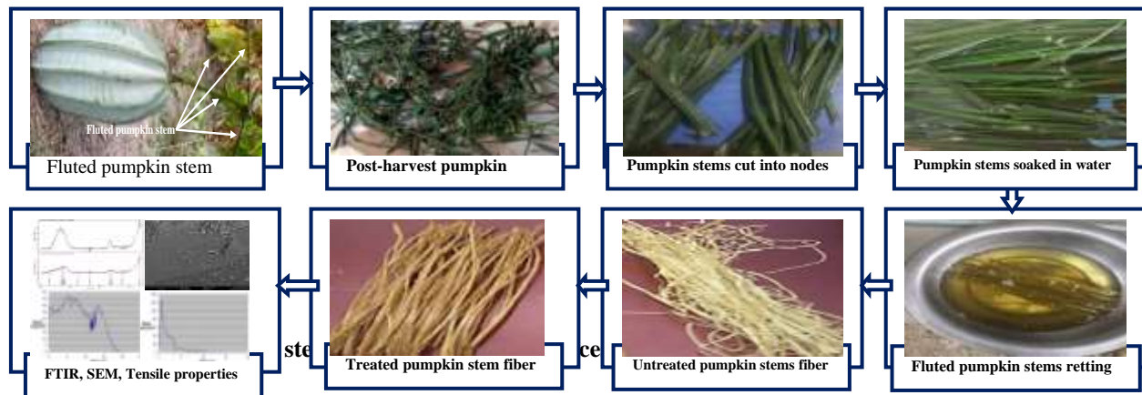
Figure 3.1: fluted pumpkin stems development and extraction process
