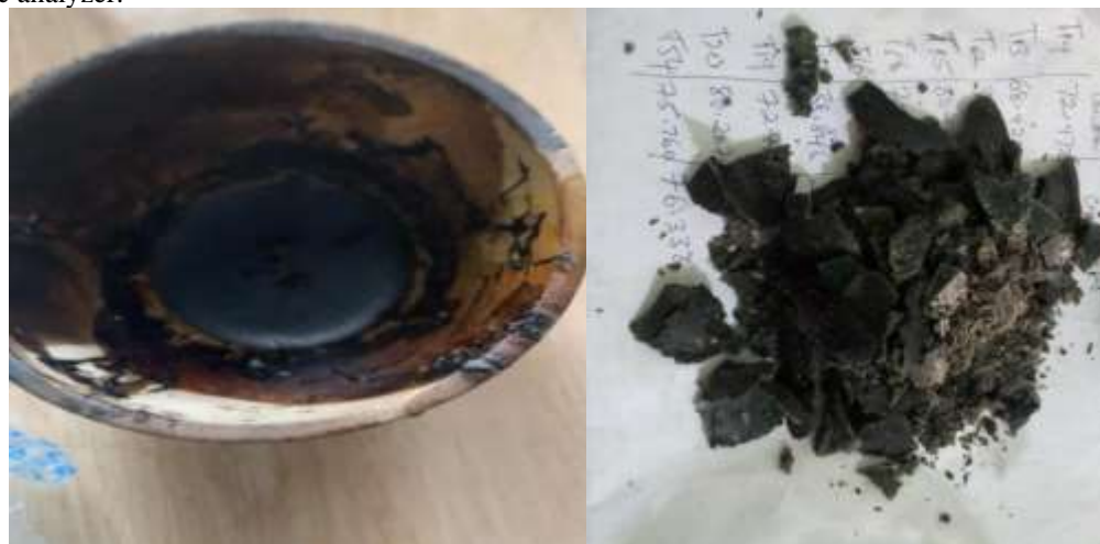
Fig 3: Polyethylene wax recovered from pyrolysis of waste sachets from sachet water industries
