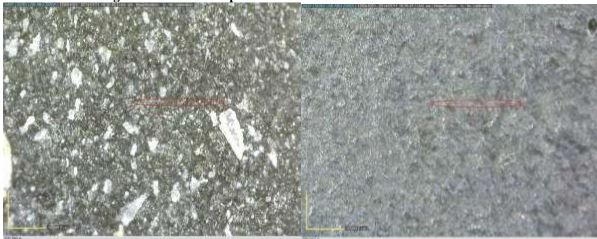
Figure 7: SEM of wax produced at 350°C a. Fracture form b. Surface form
