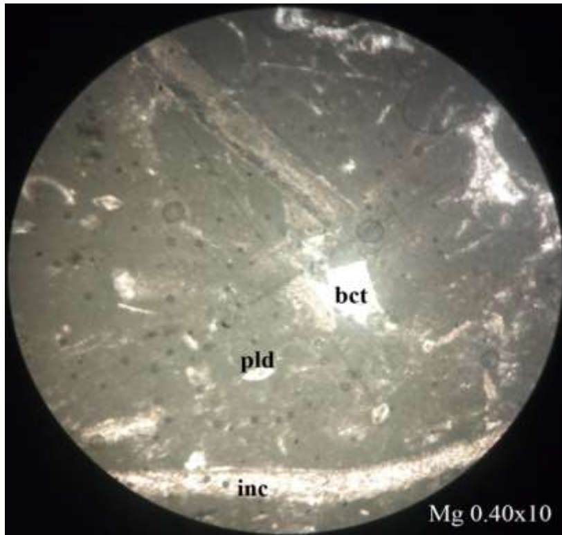
Fig. 10: Thin-section showing bioclasts (bct), peloids (pld), and intraclasts (inc) (Locality 2: 13° 32' 36" N, 05° 41' 22" E).
