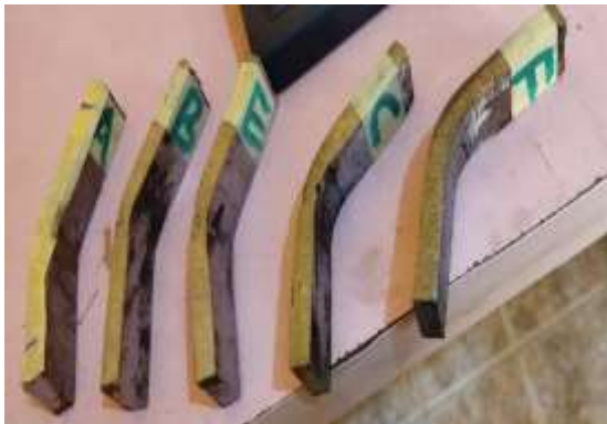
Fig 1.5. Mild Steel Sample after Testing
