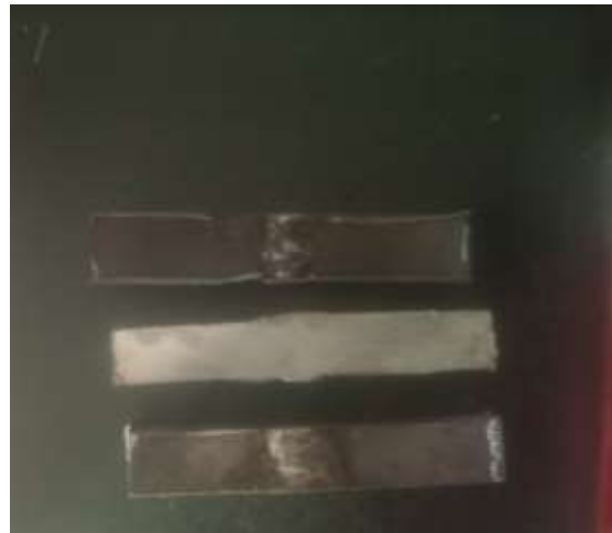
Fig 1.4. Welded Mild Steel Sample
