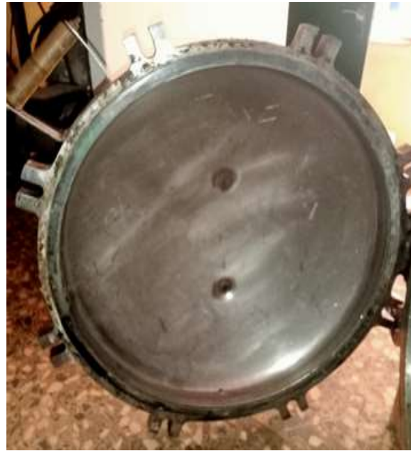
Fig. 5. Autoclave lid with improvise V-belt gasket
