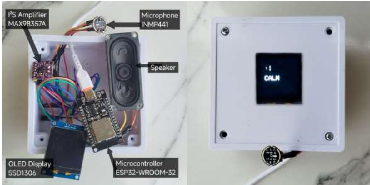
Plate 1: Physical implementation of the system showing internal and external module wiring
