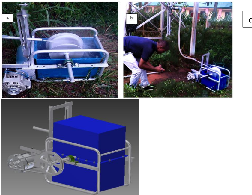
Fig. 3: (a) CFT system in operation (b) Measurement of runner shaft speed with a digital tachometer (c) Computer-aided design model of the CFT system
