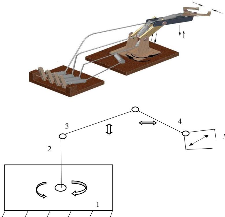
Fig 6: The model and skeletal diagram of the robotic arm
