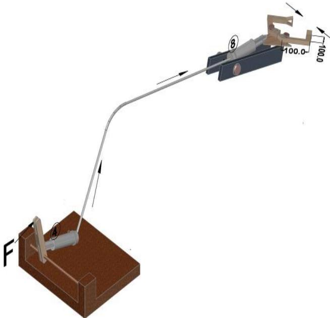
Fig 5: Movement of the Jaw
