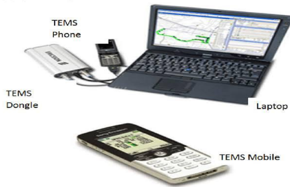
Fig. 1: TEMS Measurement Tool used for Field gathering of RSSI Data
