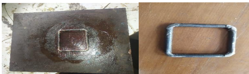
Figure 1: Fabricated mold and spacer
