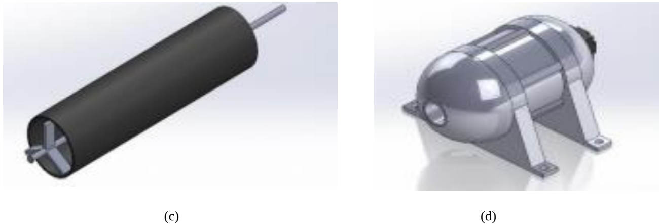
Figure 1: (a) The modeled graphics of the bitter leaf washing machine and its component: (b) washing chamber, (c) washing drum, and (d) electric motor
