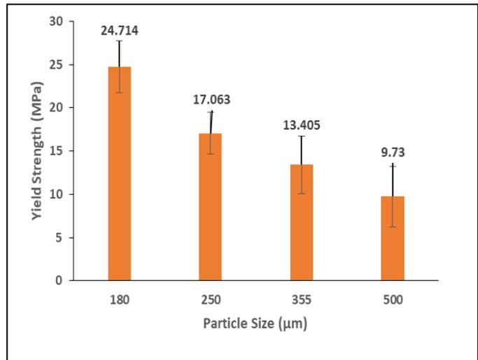
**Figure 5:** Yield strength and particle size
