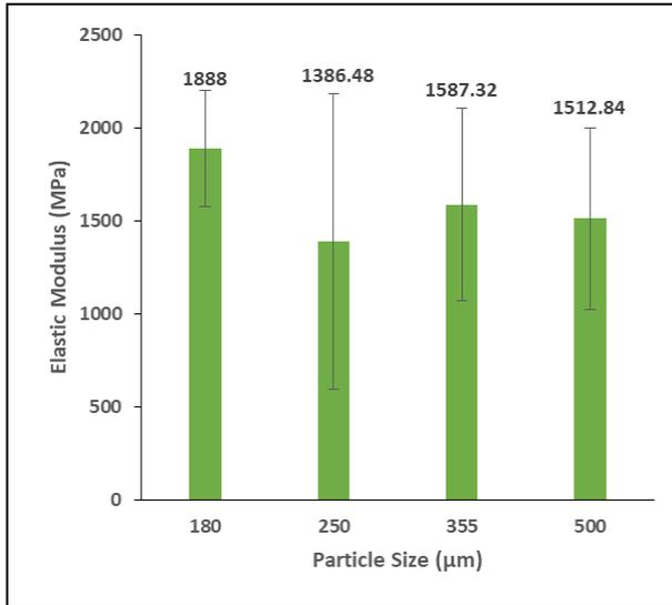
Figure 6: Elastic modulus and particle size
