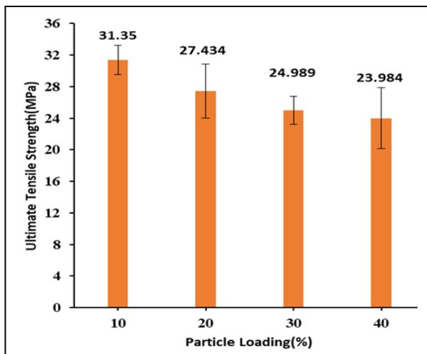
Figure 8: Ultimate tensile strength and particle loading
