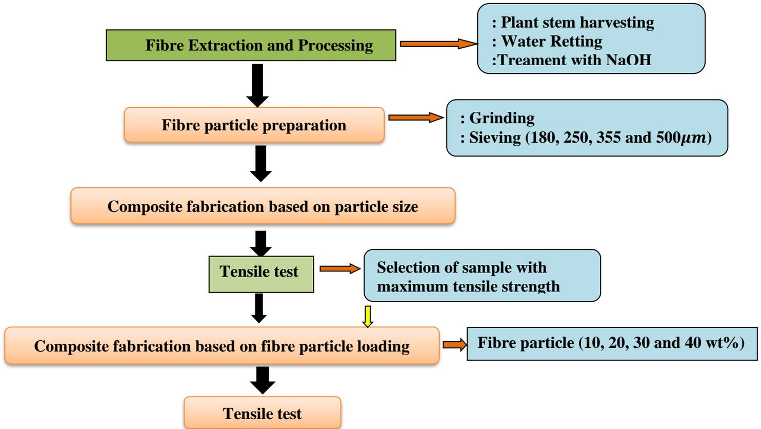
**Figure 3:** Schematic diagram of the steps for extraction, fabrication and tensile testing
