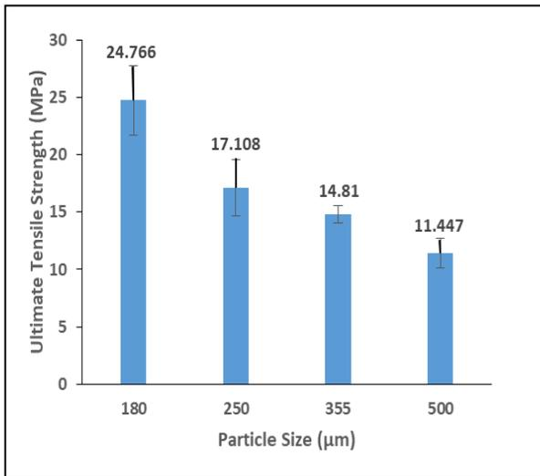
**Figure 4:** Ultimate tensile strength and particle size
