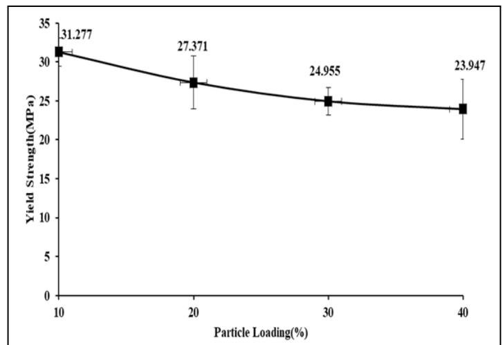
Figure 9: Yield strength and particle loading
