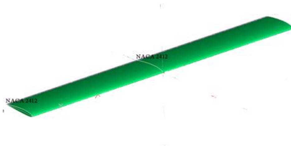
Figure 8: Wing and Plane Design with Mesh Generation of the Optimized Shape and Structure of NACA 2412 Aerofoil
